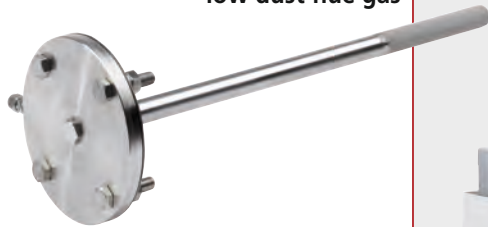
Stainless steel probe up to 900 °C with flange DN 65 PN 6 with sintered metal filter 3 μ
